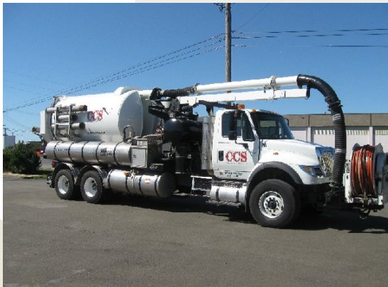
Through the use of their combo truck/sewer cleaner pictured above, CCS is able to perform utility locates through hydro excavation – a process in which pressurized water & a vacuum source are used to loosen & remove soil in a non-destructive manner.
